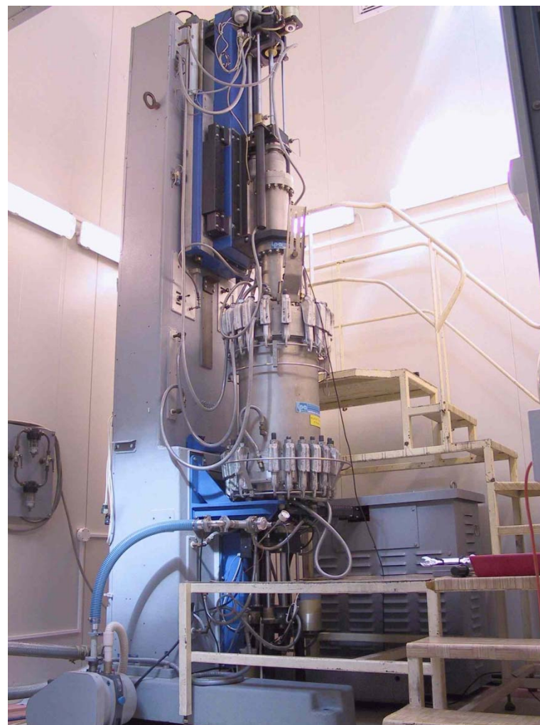
Czochralski apparatus at U. of Warsaw
