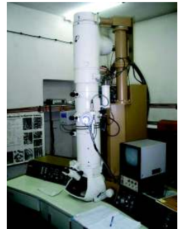
Jeol 2000EX IFAPM from 1989 200KV 0.27 nm Lab6 catode
